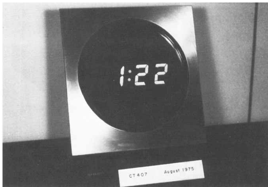
FIGURE 15 A clock which is designed to appear in the mirror using DSM.
