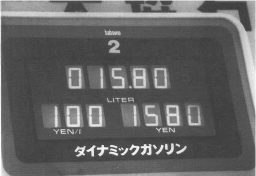
FIGURE 22 A gasoline pump meter using DSM.
