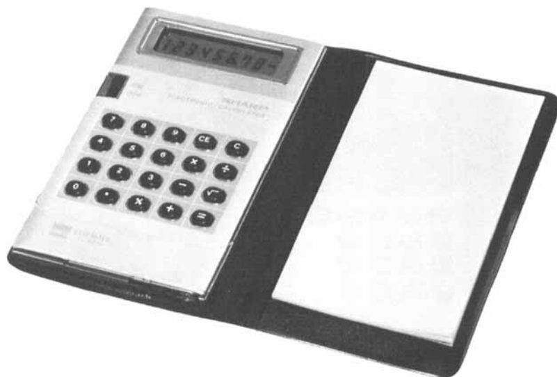
FIGURE 8 A pocketable calculator with a TN-FEM-LCD.
