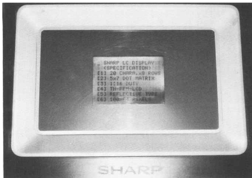
FIGURE 26 A character display using data electrodes partition.
