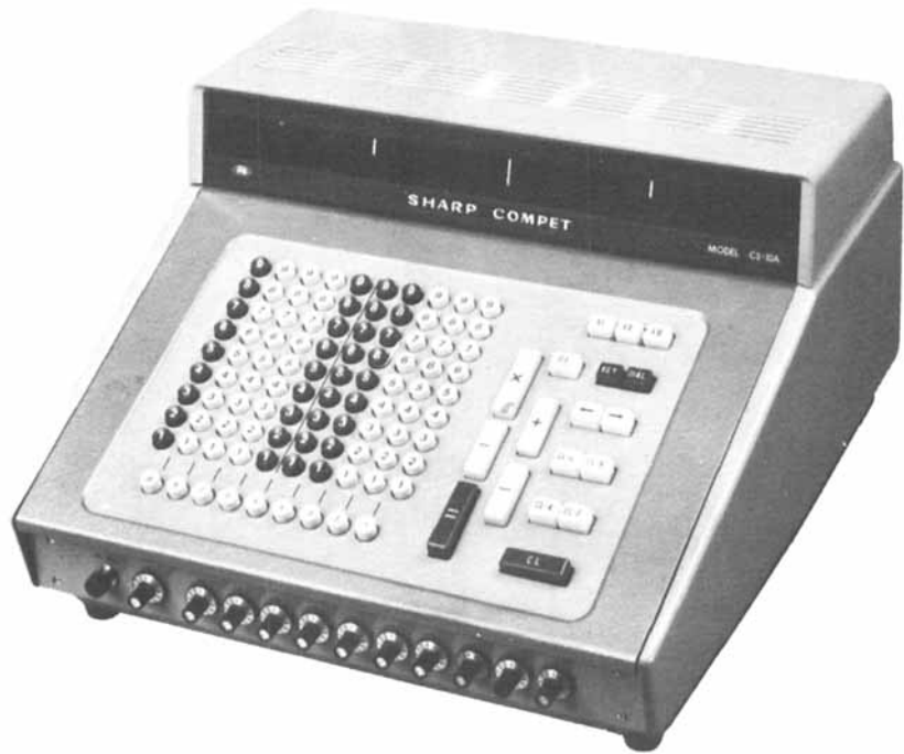
FIGURE 2 The first desk-top calculator using solid state active devices.
