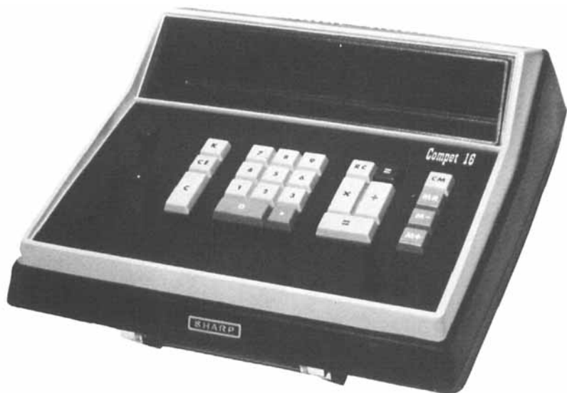
FIGURE 5 A calculator using MOS-IC's.
