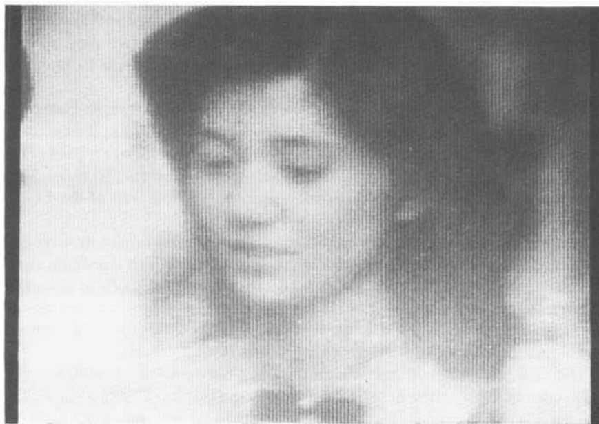
FIGURE 24 A TV image using the double matrix electrode LCD.
